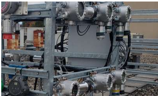
Fig. 3. Test areas at MSA provide an open air environment that serve as the primary range for sensor test operations.
